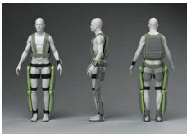
Figure 1: The ReWalk™ device from three views. The back pack holds the battery. Crutches required for stability are not displayed.
